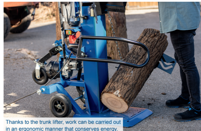
Using the log fixing device, the log can be secured before the splitting process without having to hold it.
