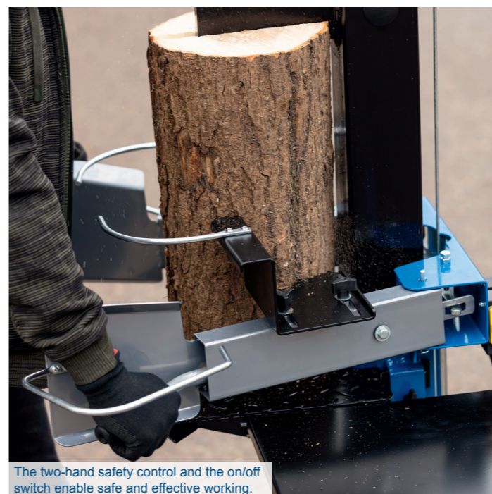
The HL810 effortlessly splits wood with a diameter of 300 mm.
